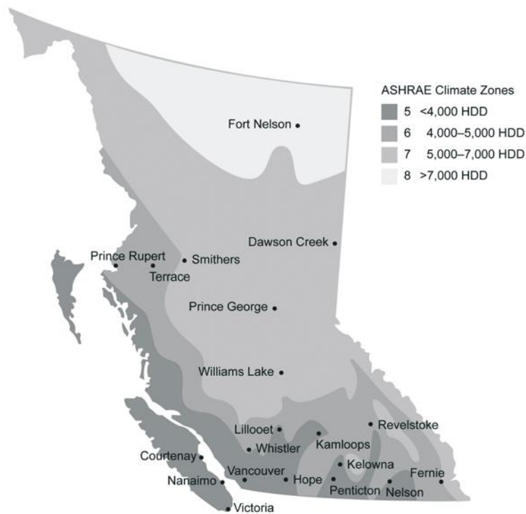
ASHRAE 90.1 Climate Zones for British Columbia. Actual Heating Degree Days (HDD) for most municipalities in British Columbia can be found in Appendix C, Division B of the BC Building Code.
